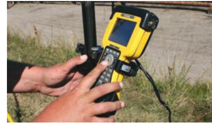
Trimble Field Computer - “Data Collector”
