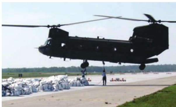
Chinook helicopter hooking up to large sand bags at the Houma Airport - 2008
