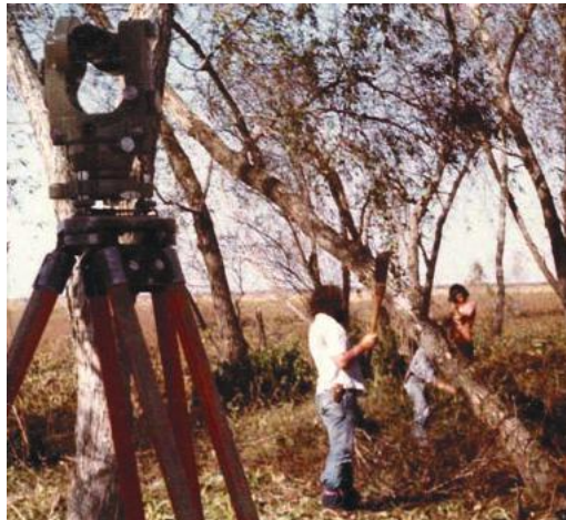
TBS instrument man and rodman "cutting line" with their sweepers through the marsh
