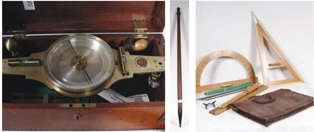
Some of Baker's survey tools: Compass, jacob staff and drawing instruments
