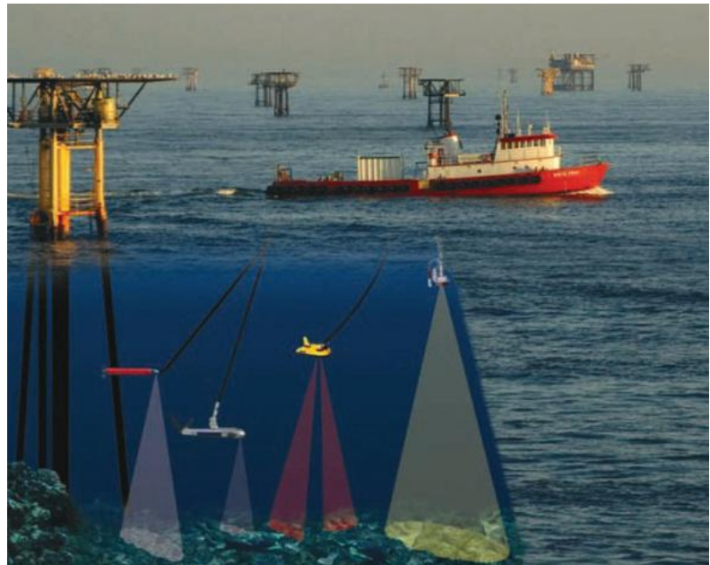
TBS Offshore Geophysical Survey Vessel utilizing Multibeam, Sub-bottom Profiler, Sonar, and Magnetometer
