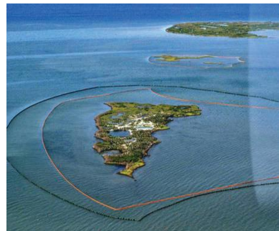
Floating Boom Placed around a Coastal Island to prevent oiling
