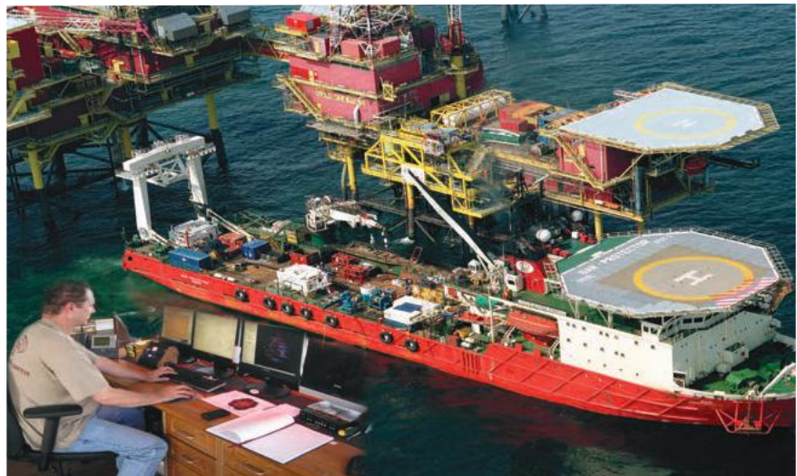
Marine Positioning - Dive vessel being positioned next to a platform in the Gulf of Mexico
