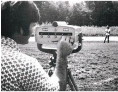
TBS Instrument Man running a HP Distance Meter with the Rod Man holding the prism target in the foreground
