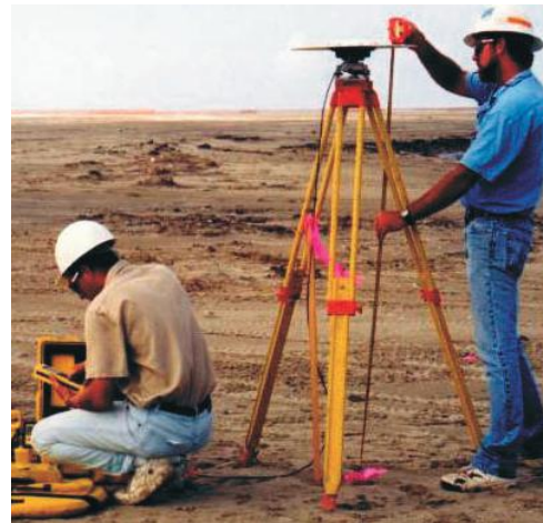
Surveying - Land based GPS survey
